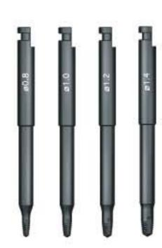
This is an instrument to remove the fractured screw by inserting the screw remover suitable for the hole formed by a reverse drill and turning counterclockwise at less than 80rpm. Screw Remover is designed with the taper structure so that the more it turns the ore the friction force required to loosen increases.
